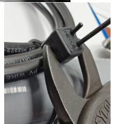
To reuse insert wire in either hole on the side of the part marked "INSERT" ensure a minimum .25" (6 mm) tail is present on the opposite side then pull back slightly to lock in place.
