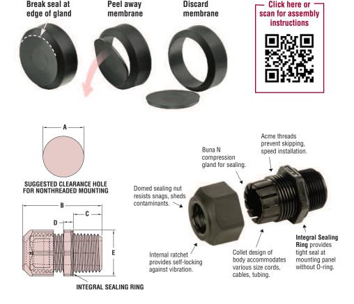
Nylon 6/6 with TPE Sealing Gland Flammability Rating 94V-2 Standard
