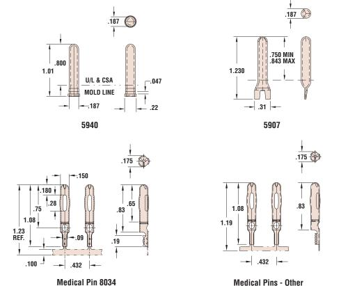
Materials Alloy 260 Brass (70% Cu, 30% Zn. Higher Cu content resists dezincification Post-Ni = Brass, Nickel plated after stamping
